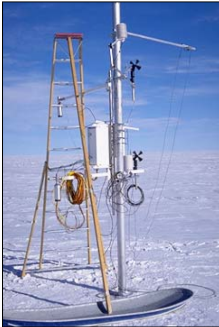
INSTALLATION OF TUNU-N AWS (LEFT), AND INSTRUMENT BOX (RIGHT)
